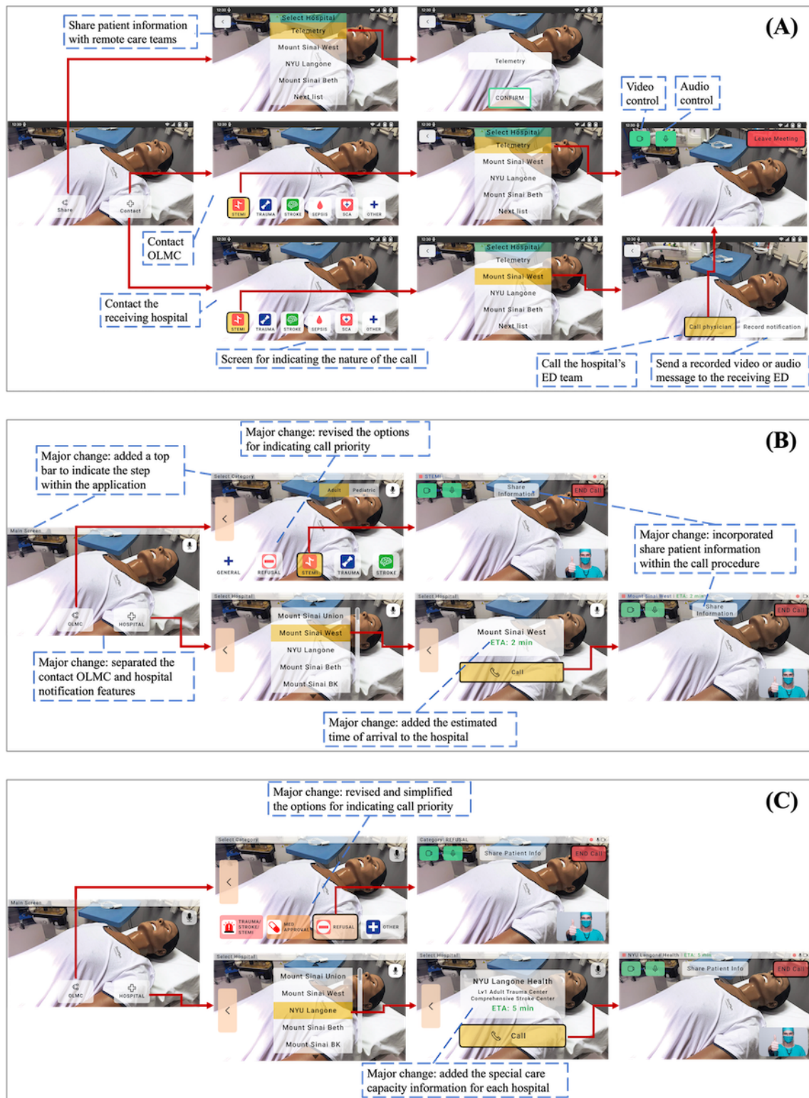
Figure 4. Iterative design of the smart glass application. (A) The first major application version created and tested in phase 1. (B) The second major application version created and tested in phase 2. (C) The final design of the smart glass application. ED: emergency department; ETA: expected time of arrival; OLMC: online medical control.
