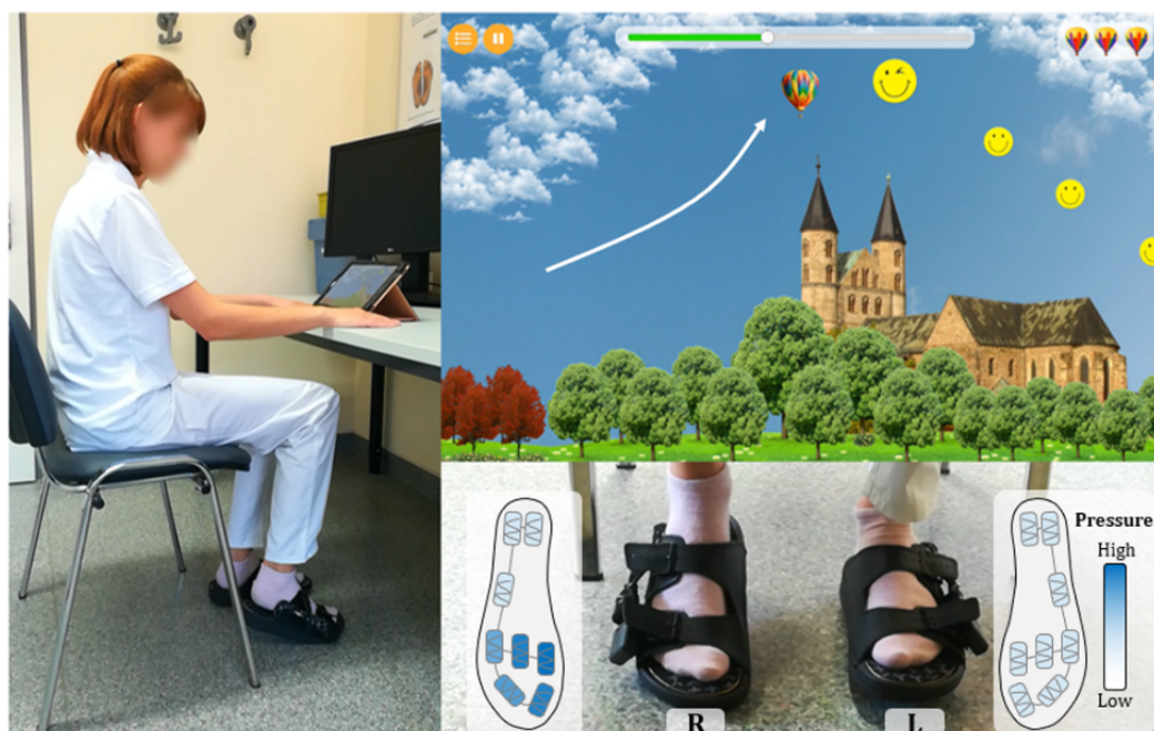
Figure 3. Visualization of the gaming session setup (Balloon Flying). The study participant is instructed to wear a pair of size-matching slippers with pressure sensor–equipped insoles and is seated on an armless chair with hands resting on the table (left image). The insoles serve as control units for the video-based gaming application that is run on a tablet (here the Balloon Flying game image is shown in the top right). The task is to collect as many smileys as possible by modulating the plantar pressure (bottom right image).
