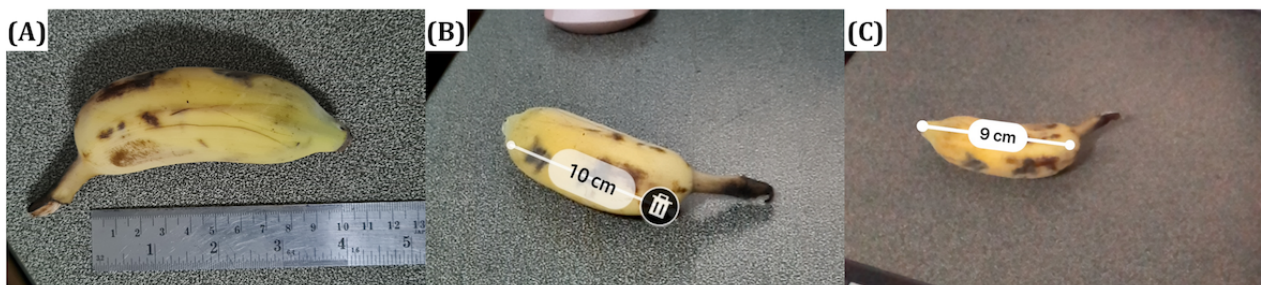
Figure 5. Measuring the size of the same banana can be done using different techniques, as shown in the figure. (A) A standard ruler is used as a ground truth measurement, (B) Samsung augmented reality Zone app, and (C) Apple iPhone Measure app. These apps use the gyroscope or accelerometer sensors in the mobile phone to accurately track the movement of the phone as the measurement line is drawn.
