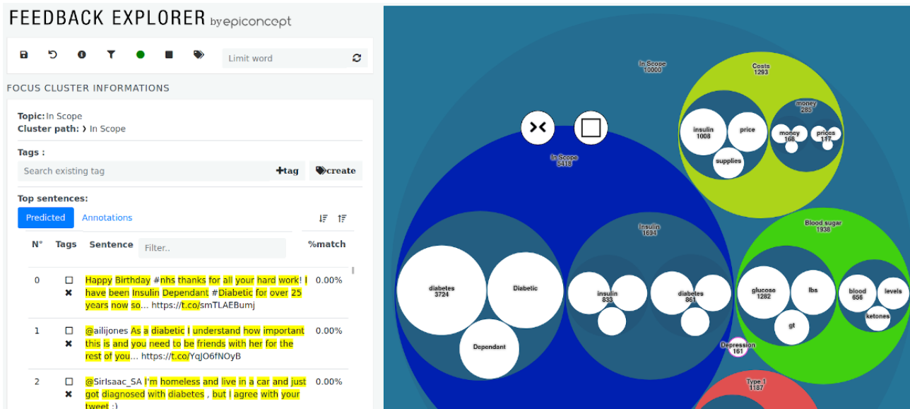
Figure 5. Visual user interface where colored circles represent user-defined topics (classifiers). Clicking on one of the nodes zooms into the node and shows the documents of the node on the bottom left. The headwords are shown in the white circles for each node.
