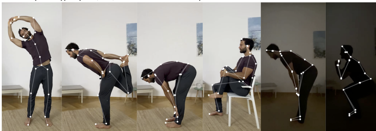
Figure 3. Examples of keypoint poses (white) inferred for various exercises by the Pose Estimation Model.
