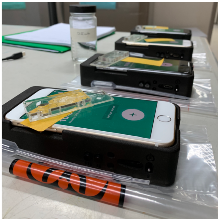
Figure 1. OmniVis rapid cholera detection device with inserted iPhone 6 and workstation setup for laboratory personnel trials.
