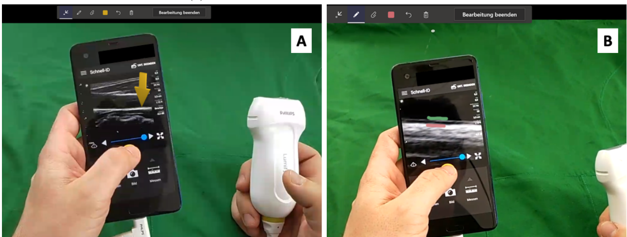
Figure 2. Examples of possible augmented reality indicators viewed while wearing the HoloLens device. (A) Arrow indicating a position to assist where to measure the intima-media-thickness. (B) Green and red lines drawn to indicate where the intima-media-thickness shall be measured.
