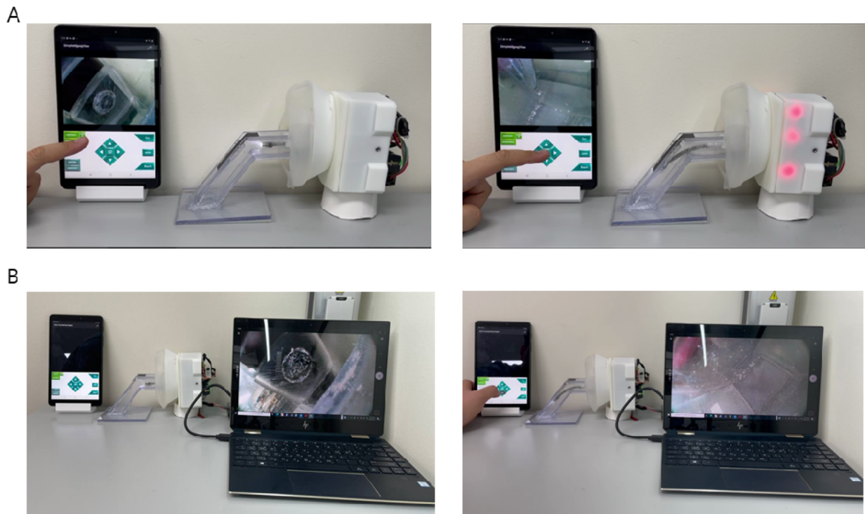
Figure 9. Wireless video transfer rate evaluation experiment. (A) Wireless and (B) wired articulation and video transfer between a contactless wireless mask endoscope and laptop computer. The transferred videos are displayed on the screens of both laptops.
