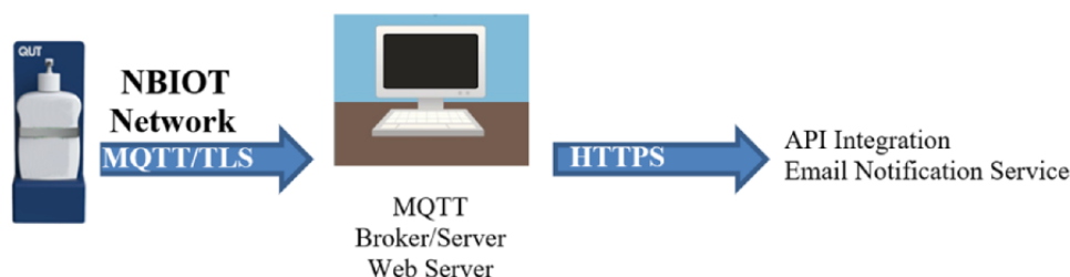
Figure 4. The process flow of data from an Internet of Things (IoT) smart sunscreen station. API: application programming interface; MQTT: message queuing telemetry transport; NBIOT: narrowband Internet of Things; TLS: Transaction Layer Security.
