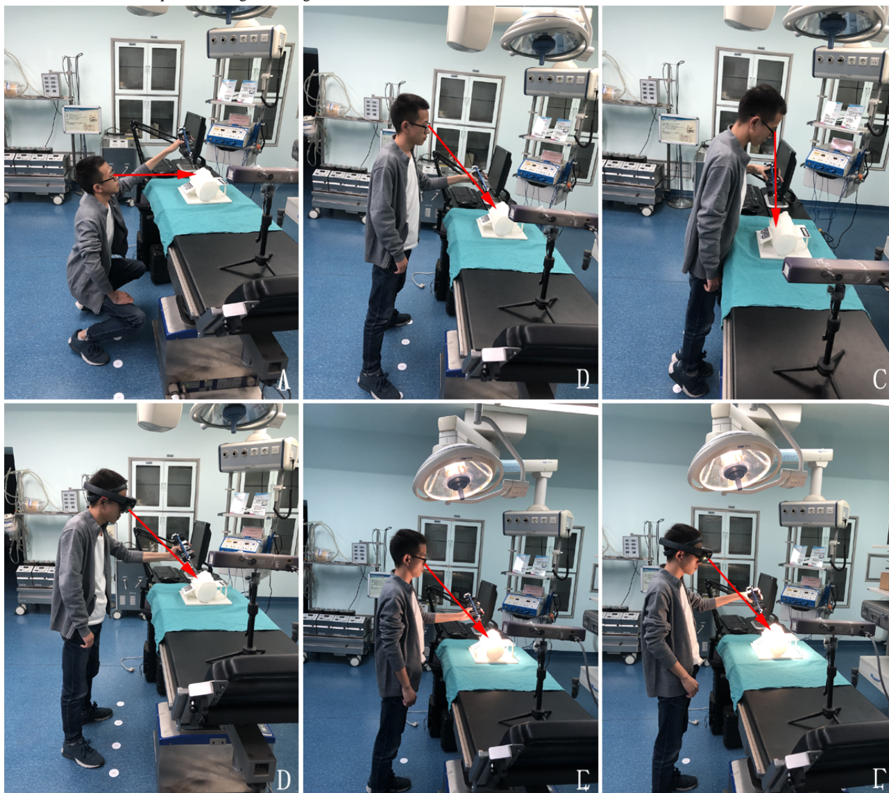
Figure 3. The coordinates of points were recorded by a tracking device (Micron Tracker) under different conditions. (A) The coordinates of points on the three-dimensional (3D) printed model were detected under the horizontal visual angle without light. (B) The coordinates of points on the 3D printed model were detected under the oblique visual angle without light. (C) The coordinates of points on the 3D printed model were detected under the vertical visual angle without light. (D) The coordinates of points on the virtual model were detected under the oblique visual angle without light. (E) The coordinates of points on the 3D printed model were detected under the oblique visual angle with light. (F) The coordinates of points on the virtual model were detected under the oblique visual angle with light.
