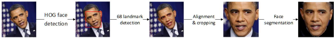
Figure 1. Pre-processing workflow to obtain chip images to use as inputs in the convolutional neural network, showing the intermediate results. Image courtesy Barack Obama Presidential Library [22].
