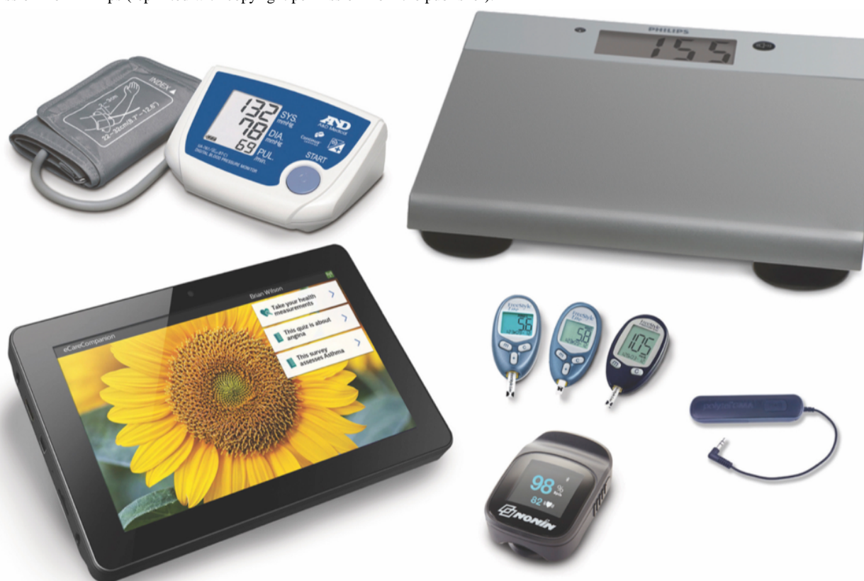
Figure 2. The Philips electronic Transition to Ambulatory Care system, featuring tablet interface and Bluetooth-enabled vital signs monitors. Reproduced with permission from Philips (reprinted with copyright permission from the publisher).
