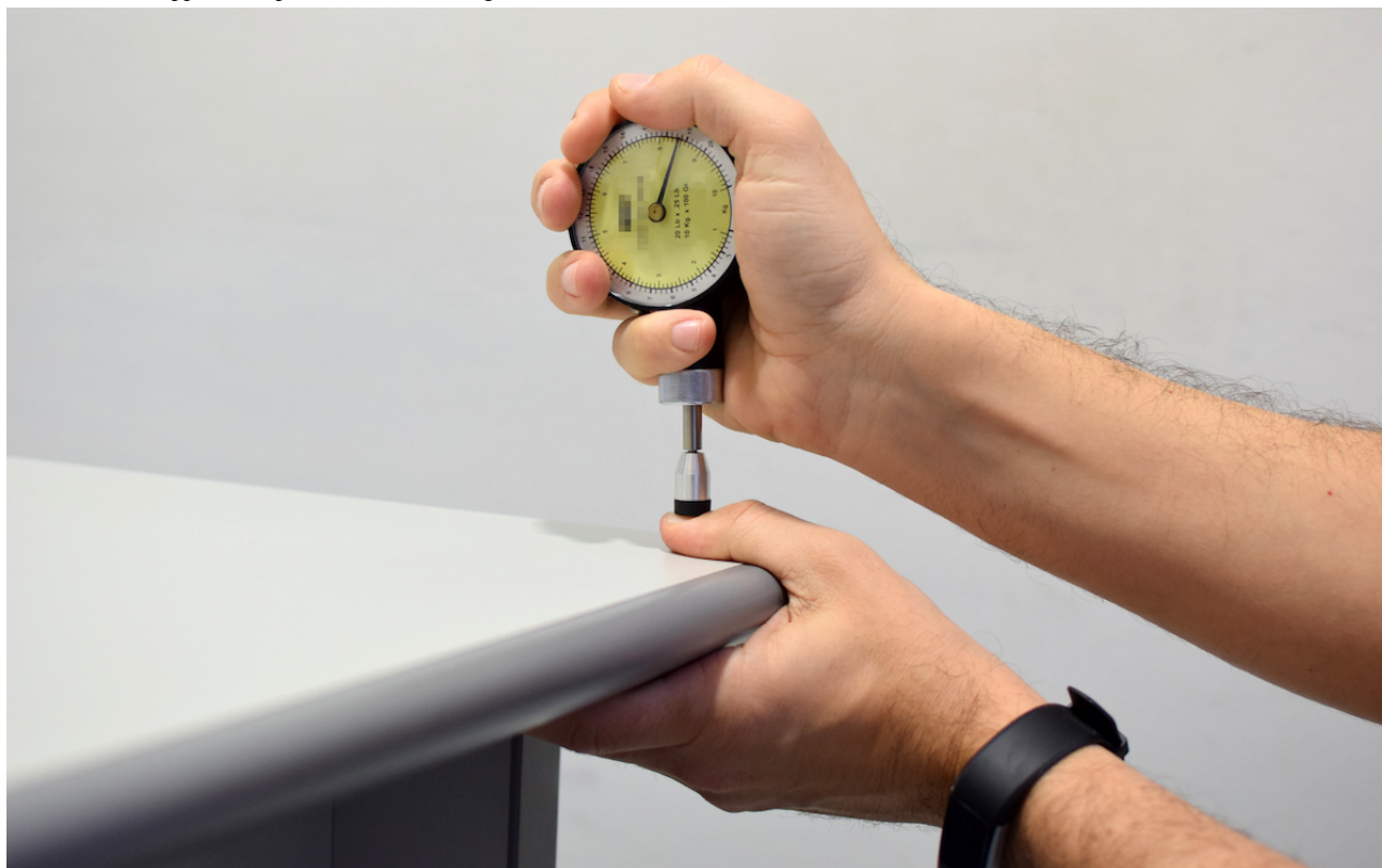
Figure 3. Pressure application procedure with the algometer.
