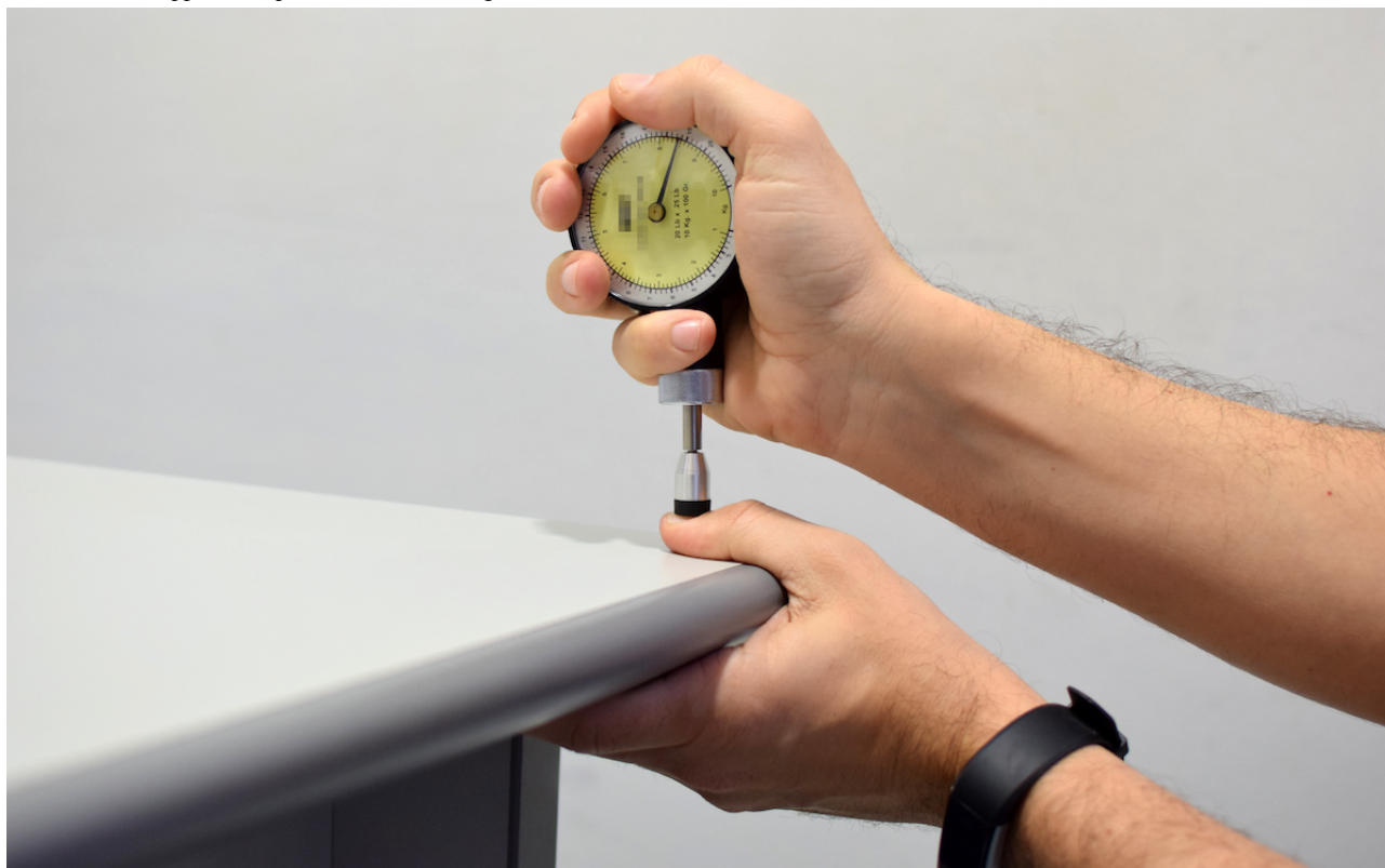
Figure 3. Pressure application procedure with the algometer.
