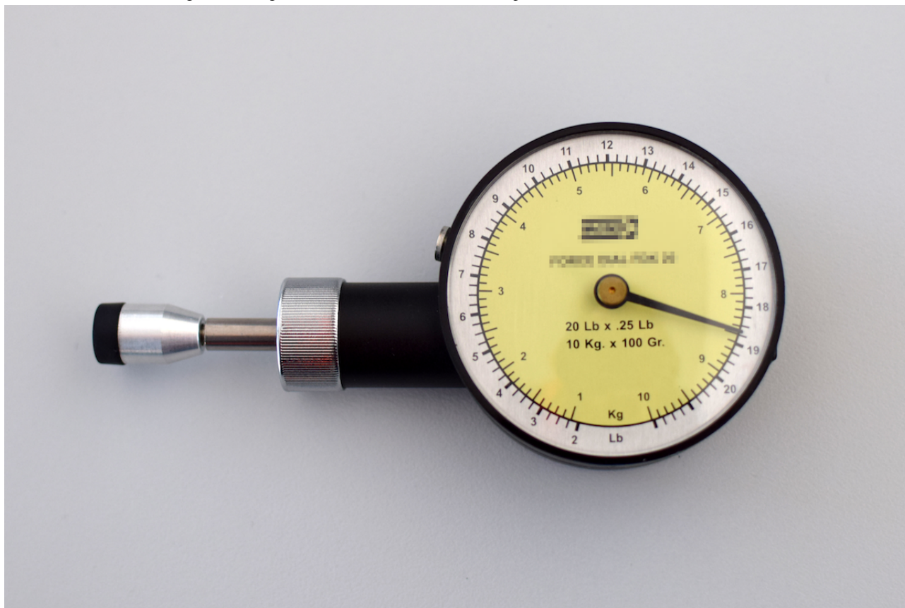
Figure 2. Force Dial FDK 20 algometer (Wagner Instruments) used to cause acute pain.
