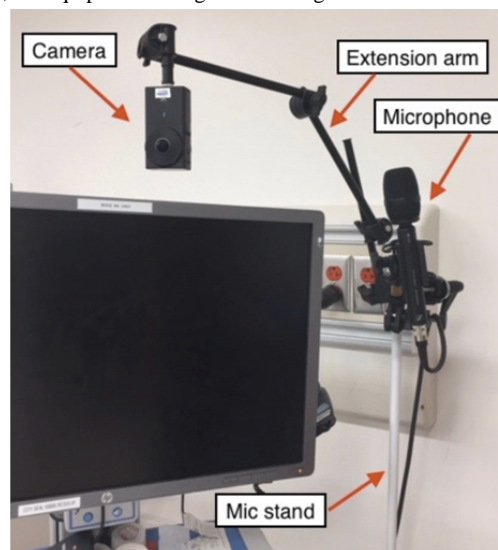
Figure 3. From the charting nurse perspective, the equipment configuration using a mic stand and extension arm.
