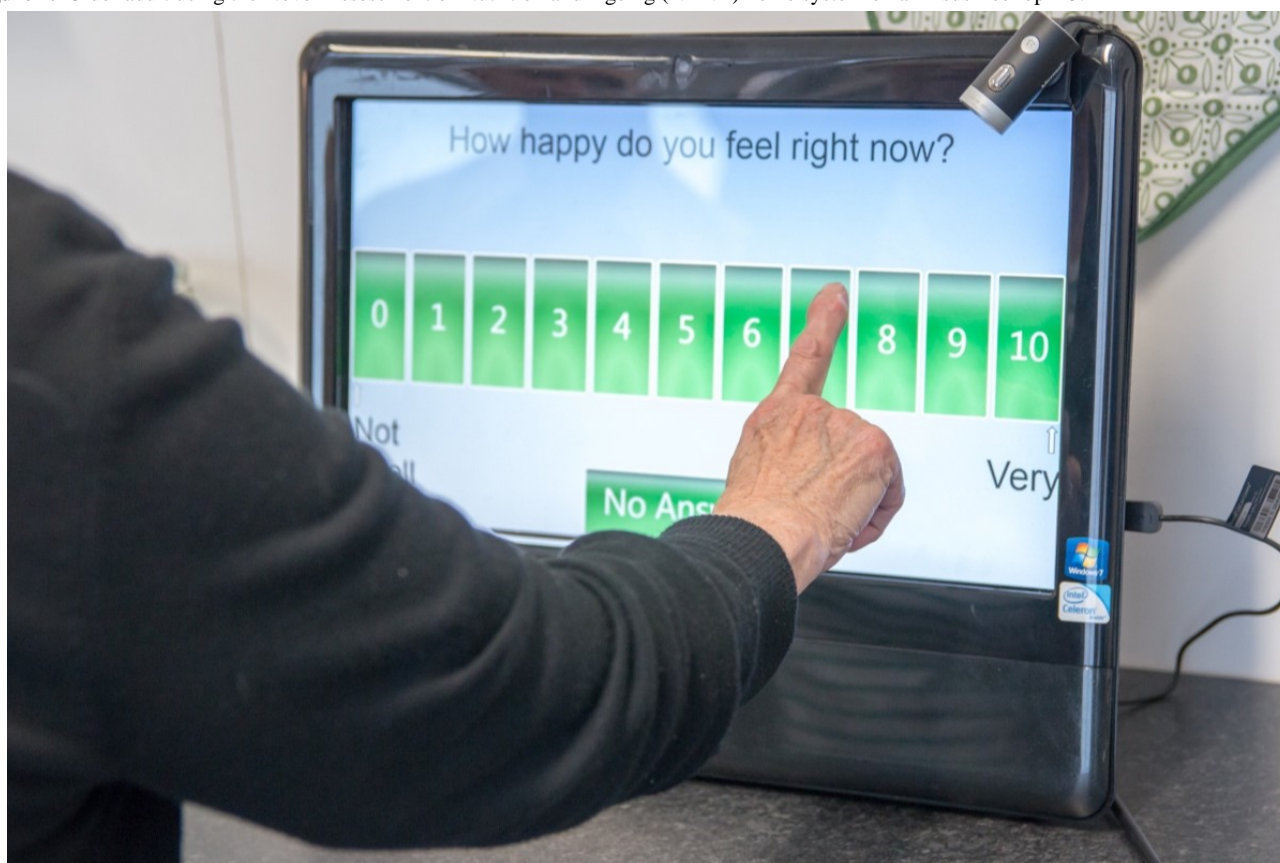
Figure 1. Older adult using the Novel Assessment of Nutrition and Ageing (NANA) home system on an Asus EeeTop PC.
