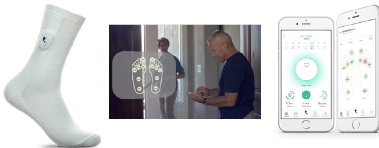
Figure 2. Typical workflow for sensor-embedded socks. The left-hand image shows a temperature-sensing sock: passive continuous monitoring of six key locations occur on the foot. The center image represents continuous monitoring: algorithms monitor temperature reading and generate alerts. The right-hand image displays the patient interface of the app, used for viewing the alerts.
