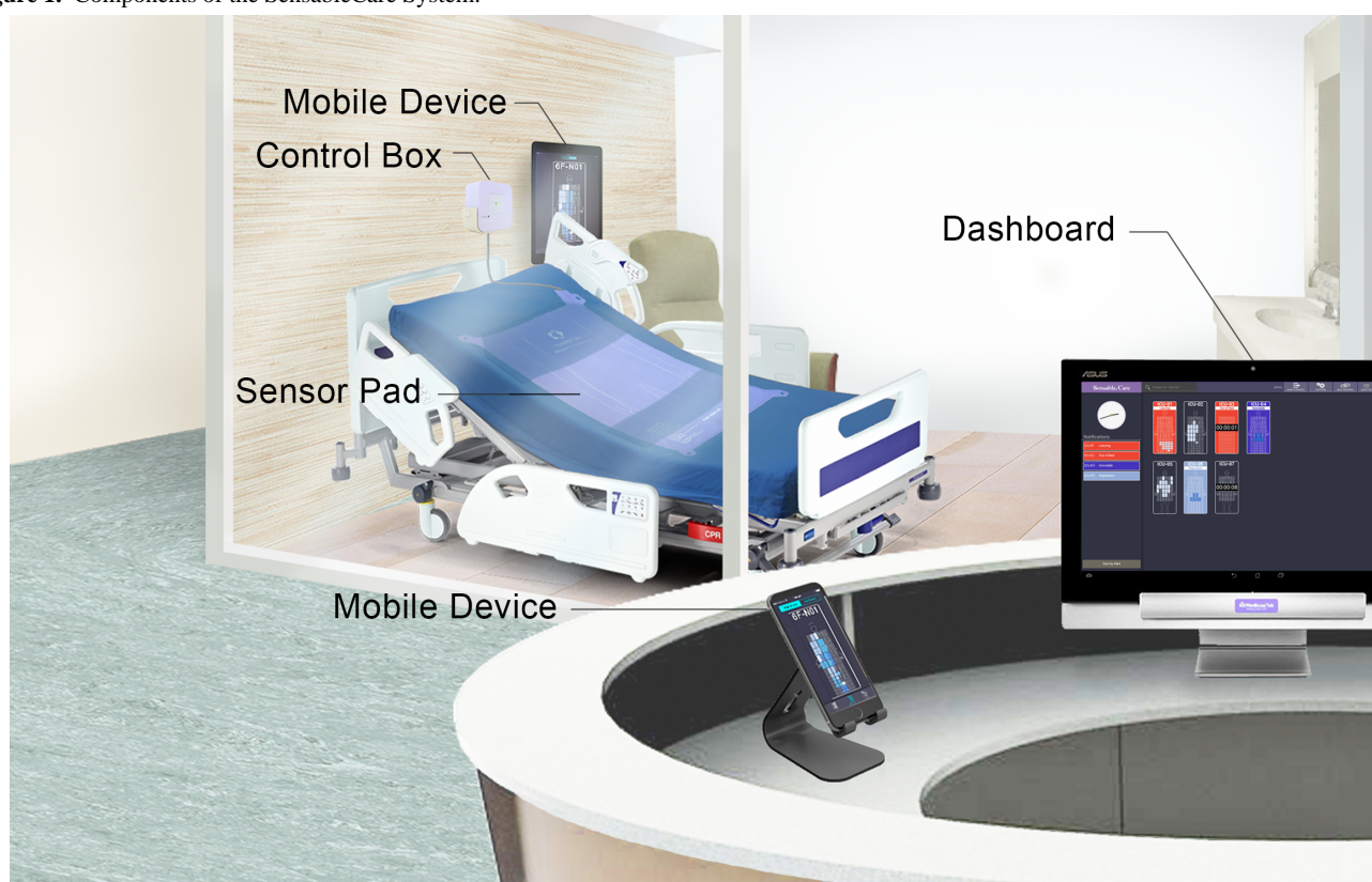
Figure 1. Components of the SensableCare System.
