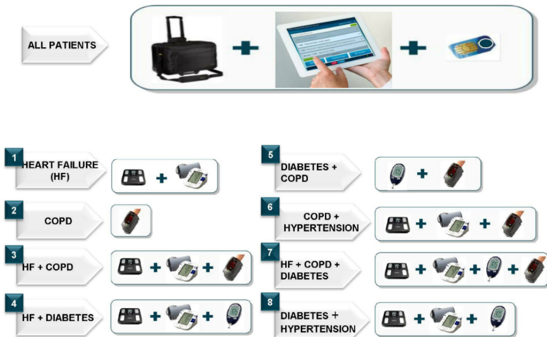
Figure 1. Telemonitoring program devices, according to a patient’s disease: scales, blood pressure monitor, glucometer, and pulse oximeter. COPD: chronic obstructive pulmonary disease.
