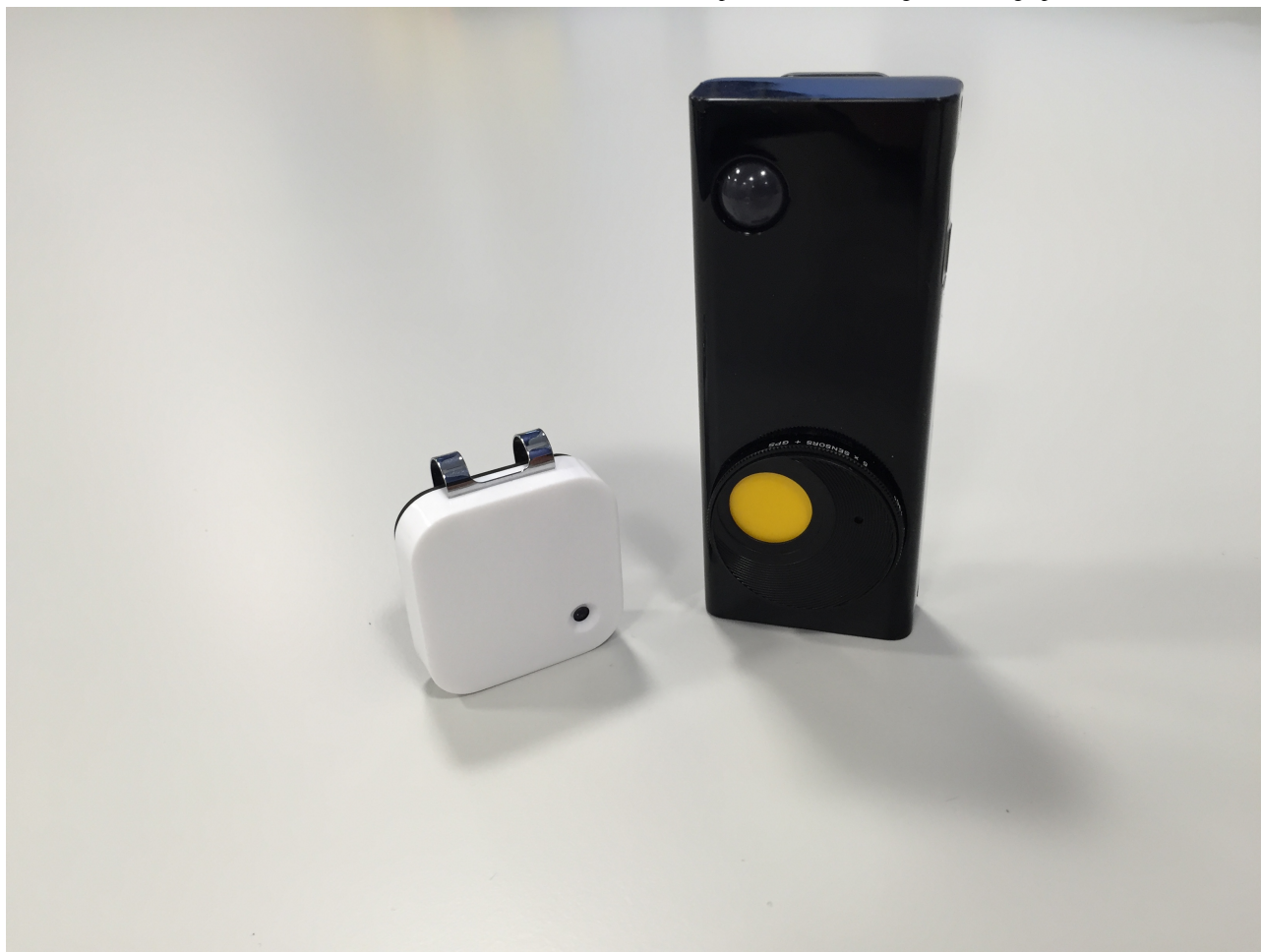
Figure 4. Hardware of two wearable cameras. Shown on the left is the Narrative clip [201] and on the right the Autographer [200].
