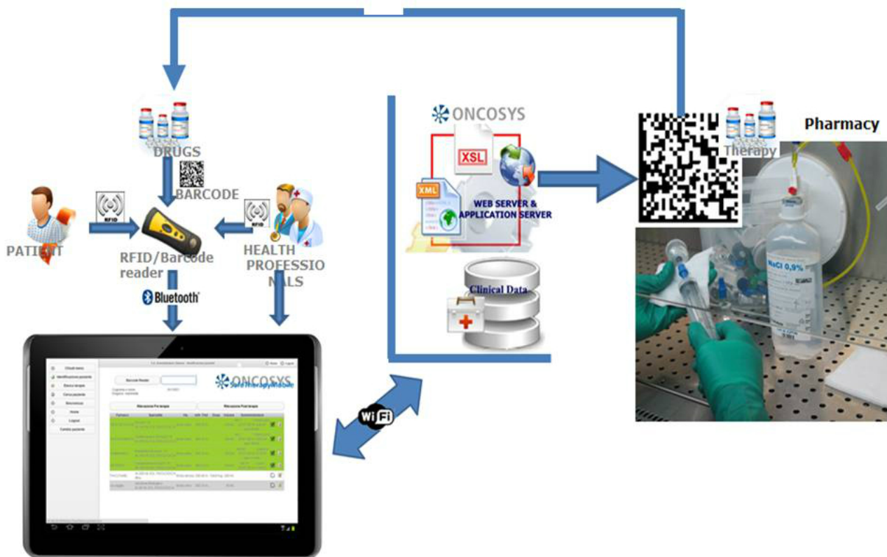
Figure 1. The basic components of the STM system. The eOPR originates a CPOE that is univocally associated with the patient's RFID bracelet and the barcodes of the individual chemotherapy and ancillary drug, and washing solution. The RFID/barcode communicates via Bluetooth with the tablet, which communicates via Wi-Fi with the server of the OPR. The RFID/barcode reader checks the patient's RFID bracelet, the nurse's RFID, and the barcode on the infusion bag before each drug administration.
