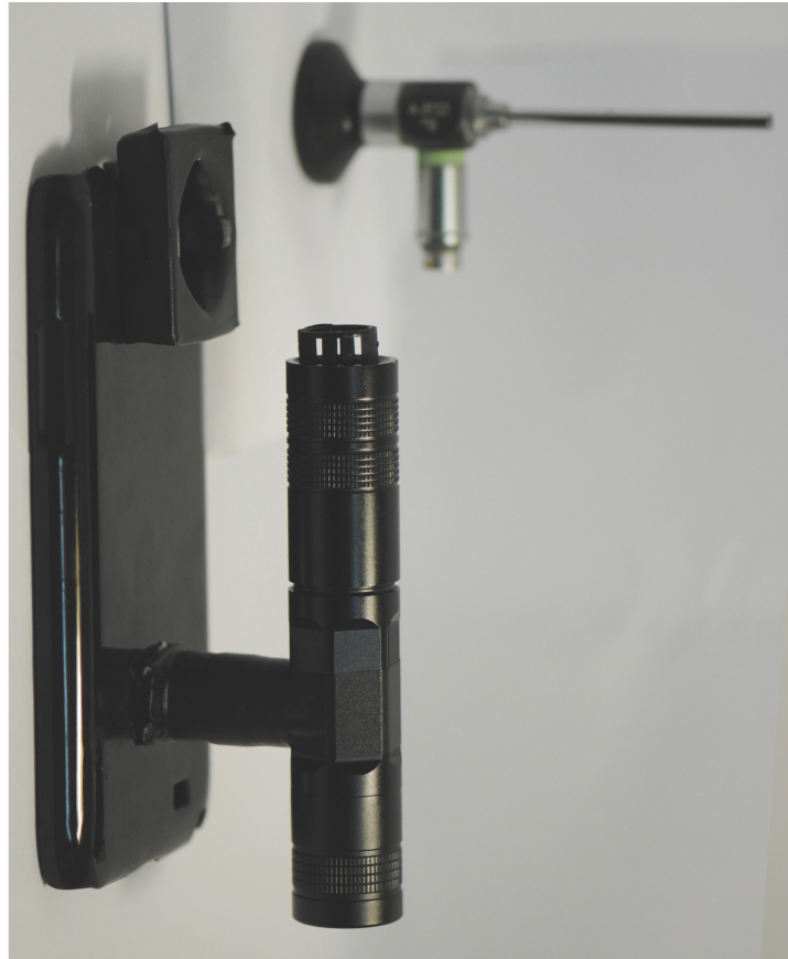
Figure 2. Self-designed specific adapter with portable light source.
