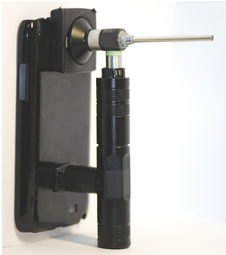
Figure 3. Prototype of a self-designed smartphone-based otorhinoendoscope.
