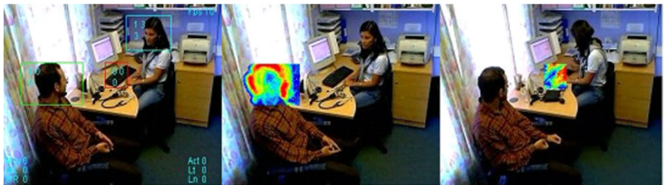
Figure 4. Measurement of nonverbal interactions using PRS, patient's head nodding and doctor's keyboard use
