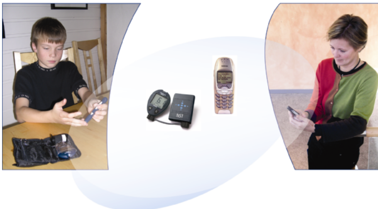
Figure 1. Blood glucose readings are sent to parent's mobile phone
